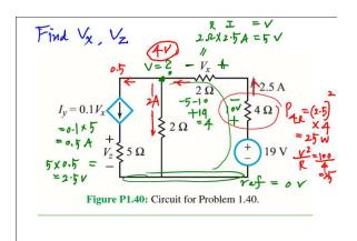
► The algebraic sum of the voltages around a closed loop must always be zero. ◀
