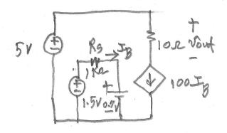
$$\frac{T_{8} = 1.5 - 0.7}{1 \text{ Ke}} = 0.8 \text{ mA}$$
