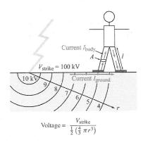
Each shoe provides some degree of protection with a series resistance of 750  $\Omega$ , and each leg has a series resistance of 500  $\Omega$ .
